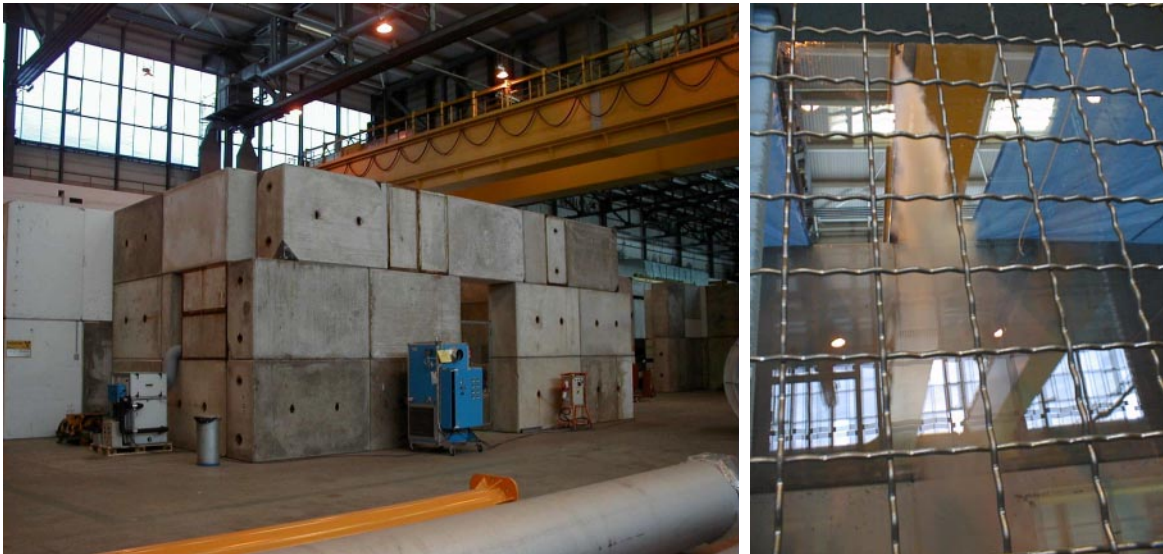
Figure 4. General layout of the experiment and spill point during a 50 l LAr/min. leak
