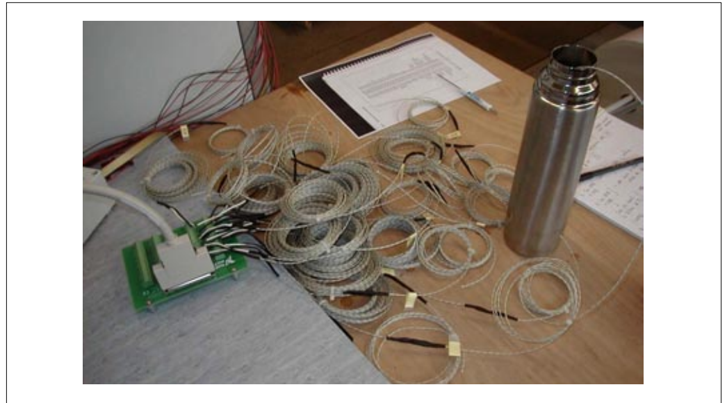
Figure 5.7 Thermocouples and Cold Junction
