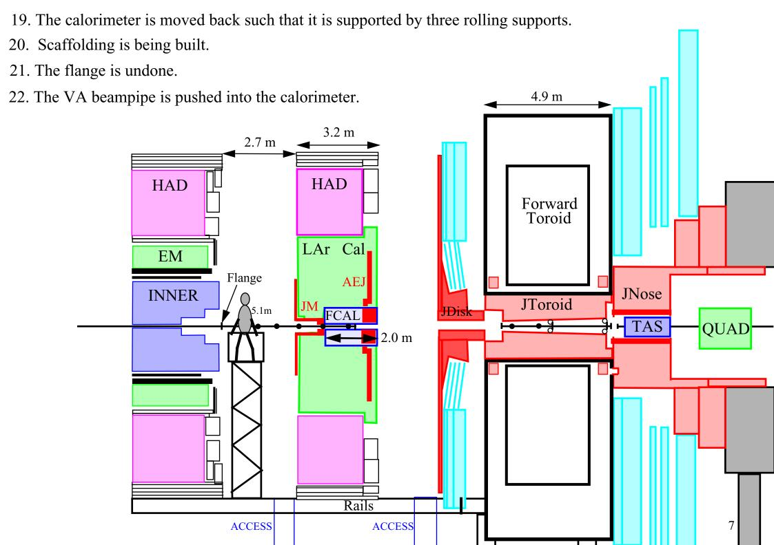
23. The calorimeter is moved furher back. 4.9 m 3.2 m 3.3 m HAD HAD Forward Toroid LAr Cal EMAEJ JNose **INNER** JToroid JDisk FCAL 5.1 m ⊢ TAS QUAD
