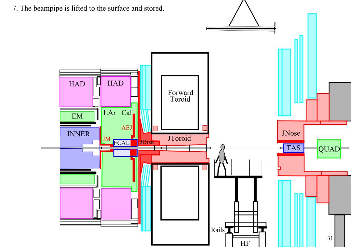
8. The two fixed supports inside the toroid shielding are unlocked (0.2h x 0.3 mSv/h = 0.06 mSv) 9. The fixed support at the end of the toroid shield is removed and replaced with a rolling support  $(0.3h \times 0.4 \text{ mSv/h} = 0.12 \text{ mSv})$ HAD HAD Forward Toroid LAr Cal Fixed support to EM be unlocked **AEJ** Fixed support to JNose **INNER** be replaced by JToroid . FCAL JDisk rolling support - TAS **QUAD** Rails I 32 HF
