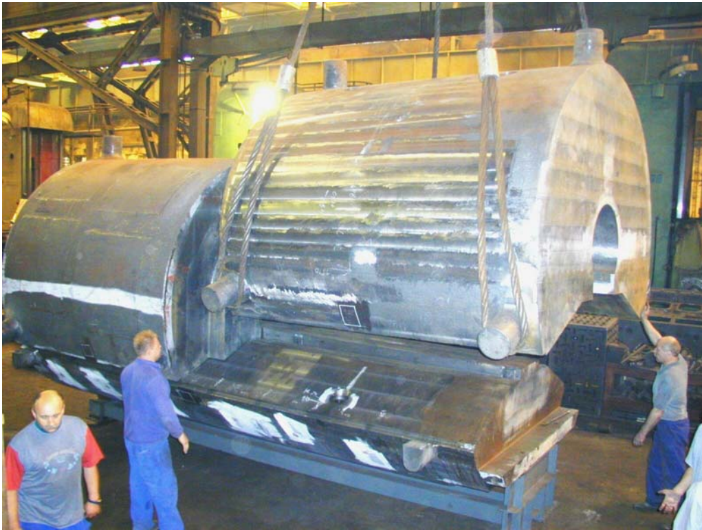
Figure 4.9 The three cast iron pieces of the JF core section during manufacturing at the Skoda factory.
