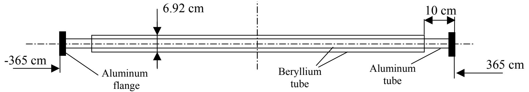
Fig. 1 Sketch of the ID Beam pipe section.
