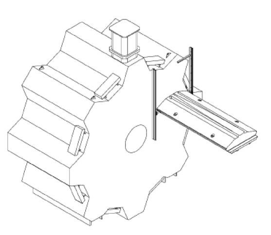
JF bridge guidance rails are attached to the rails above the toroid.
