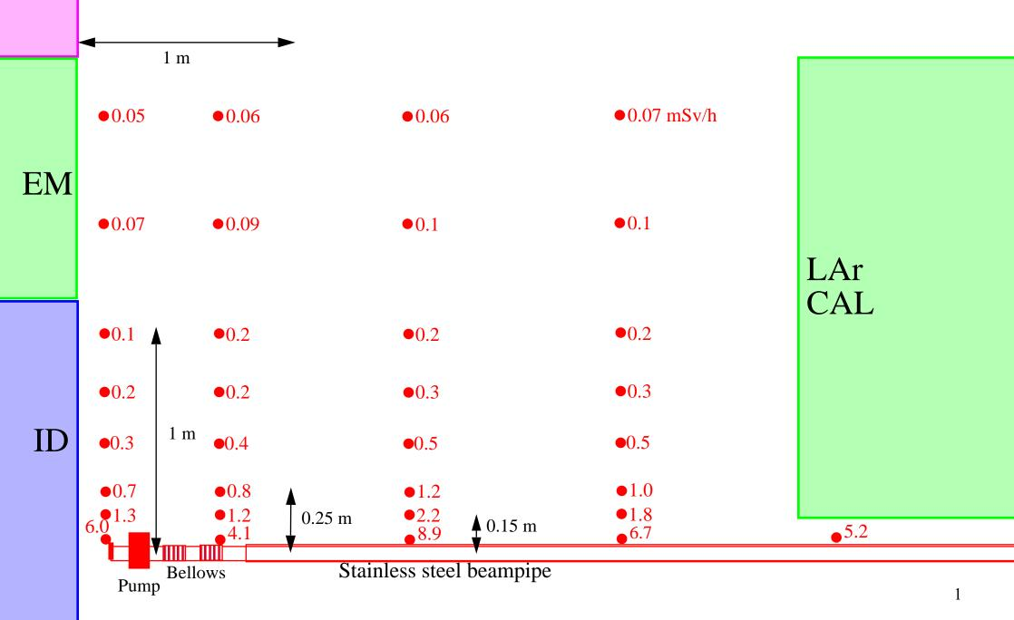
Dose rates in mSv/h from the VA beampipe after a 100 day run HAD and 100 days cooling. Calculation by M. Morev. 1 m • 0.01 mSv/h •0.01 •0.01 •0.01 EM •0.01 • 0.02 • 0.02 • 0.02 LAr CAL •0.02 •0.03 •0.03 •0.03 •0.03 •0.04 •0.05 •0.05 1 m ID •0.05 **•**0.06 •0.09 •0.09 •0.1 •0.2 •0.1 •0.2 •0.2 •0.2 •0.3 0.25 m •0.4 **♦** 0.15 m 10**0.9** 0.7 1.6 1.2 Stainless steel beampipe Bellows Pump
