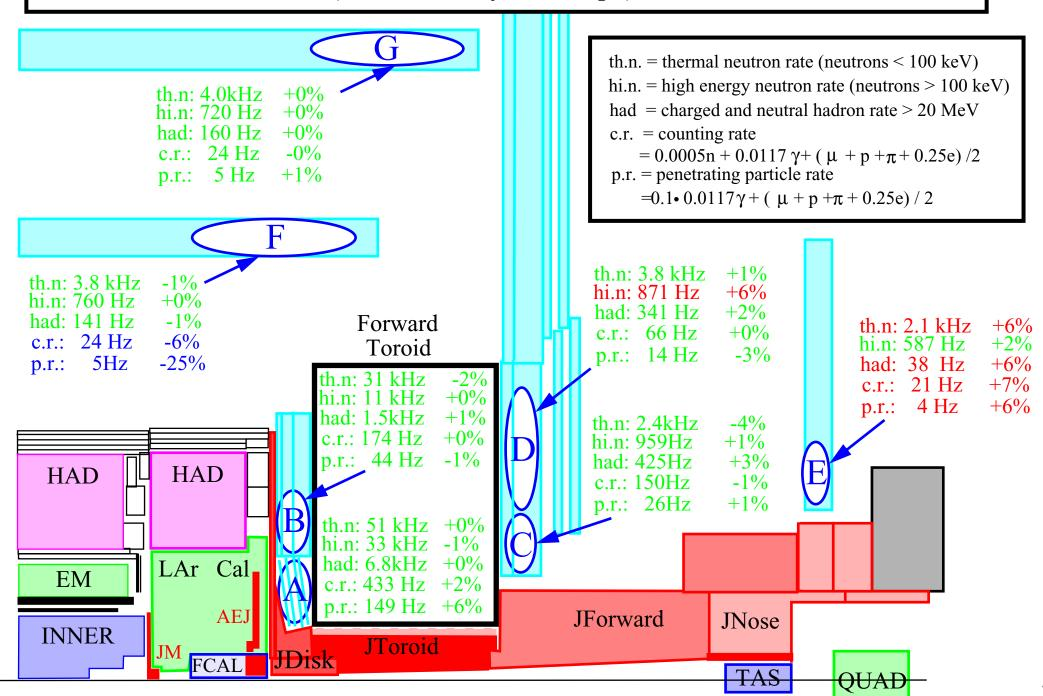
Change in particle flux if the radius of the large octagonal pieces is reduced and the front octagonal piece is removed. (Simulation by M. Shupe)
