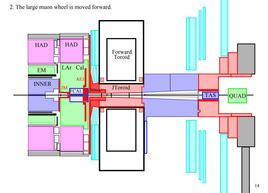
2. The large muon wheel is moved forward. HAD HAD Π Forward Toroid LAr Cal EM AEJ INNER JToroid JM FCAL JDisк TAS QUAD
